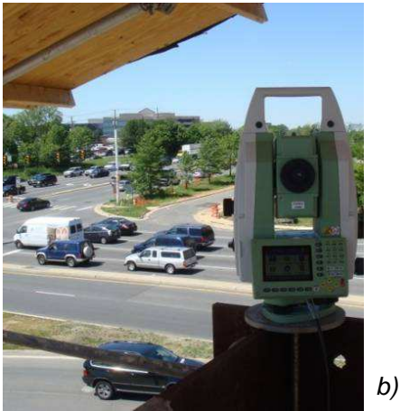
Fig. 13 a) View of the “IMZ” (dashed line) and the surface settlement monitoring points including the Virtual Points (green triangles) and b) Total Station Theodolite at Tysons Corner
