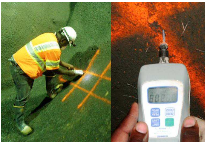
Fig. 9 Penetration Needle Test
