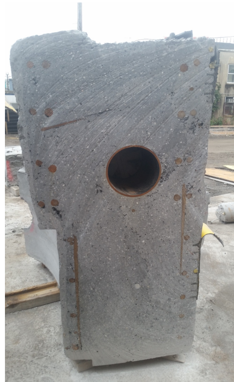
Figure 6: Encapsulation of reinforcement, embedments and encasement of waterbarrier (on right lower side)
