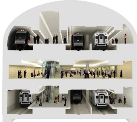
Figure 1. Trans Hudson Express (THE) station cavern New York Penn station Expansion (NYPSE) cross-section.
