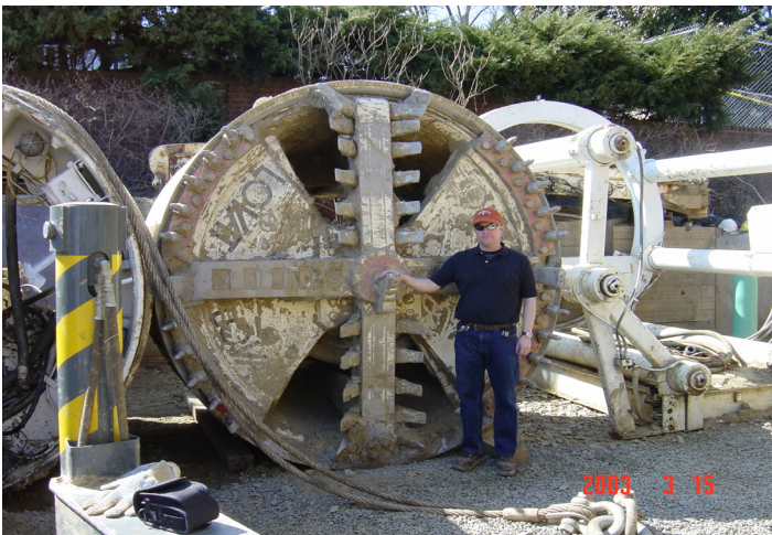
Figure 1. Soft ground TBM for the construction of steam conveyance tunnels.
