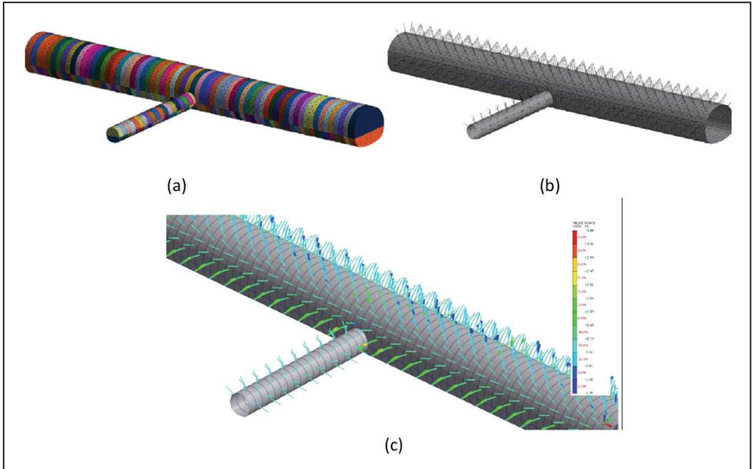
**Figure 4.** 3D Finite element model for the mined tunnel with connecting Adits: (a) model construction stages, (b) stage after support installation, and (c) axial forces developed in the rock dowels
