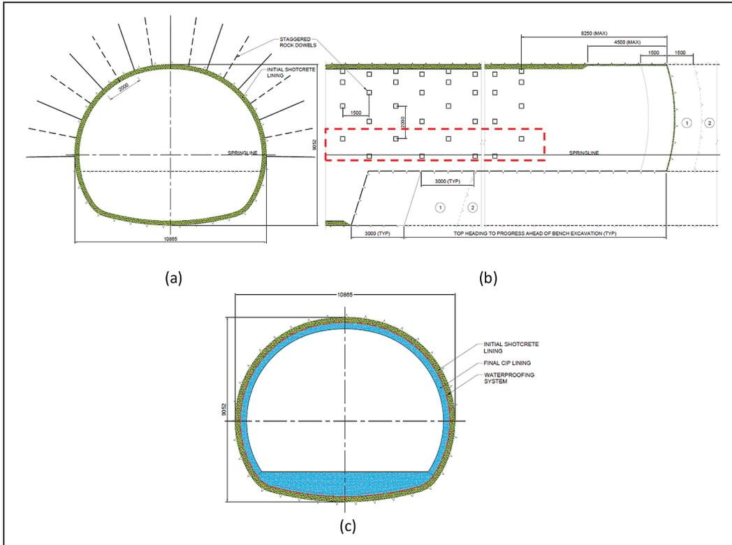
**Figure 3. Typical tunnel geometry: (a) primary lining, (b) typical excavated sequence with rock dowels, and (c) secondary lining**
