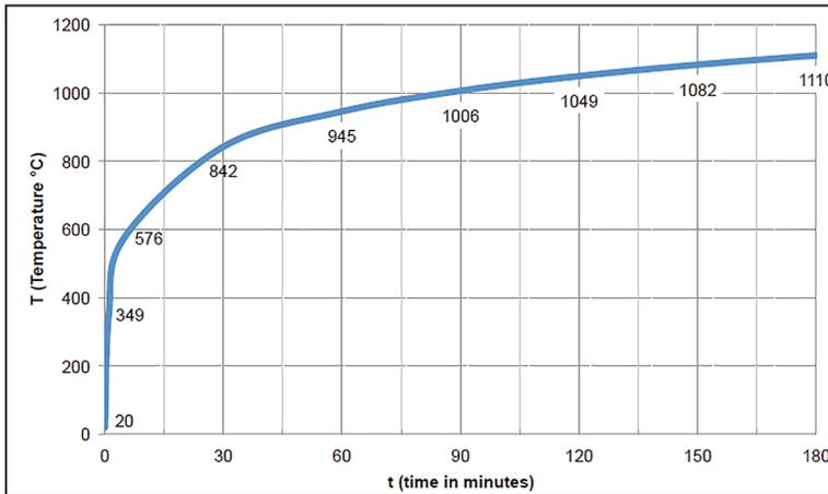
Figure 5. Standard ISO 834 temperature-time curve for a 3-hour fire duration
