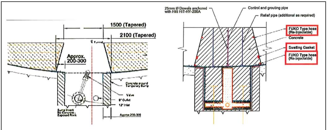
Figure 10. Front view of the temporary sump: before and after completion of final lining
