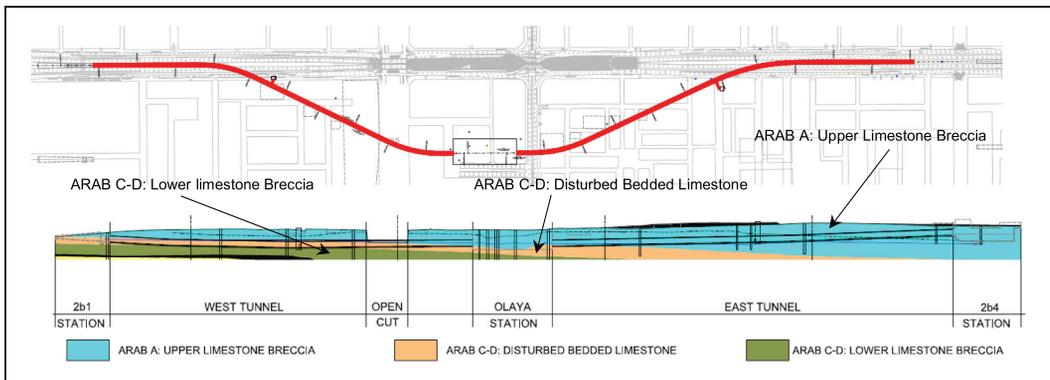
Figure 2. Mined tunnel plan and profile view with geology
