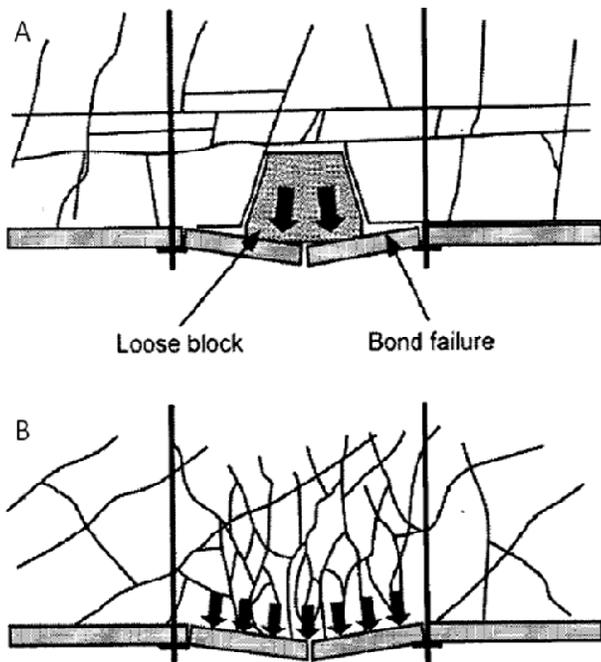
Fig. 6. Flexural failure modes due to A) loose block and B) weak rock zone from Martin et al. [15]
