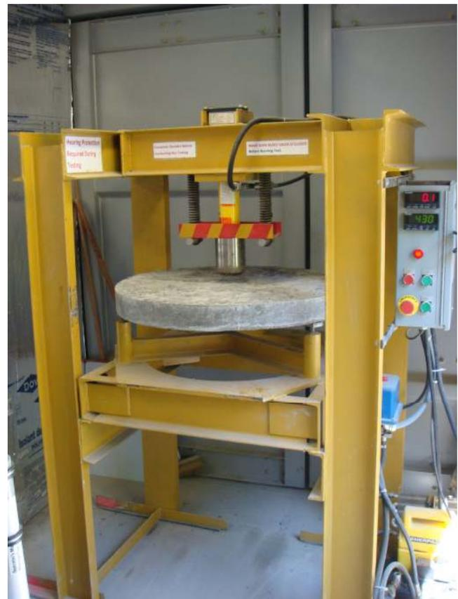
Fig. 4. ASTM 1550 test machine at Devil's Slide Tunnel with sample ready to be tested.
