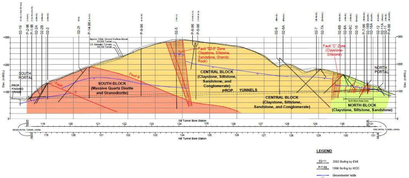
Fig. 1. Longitudinal profile along tunnels, showing South Block, Central Block, and North Block along with expected faults [4].
