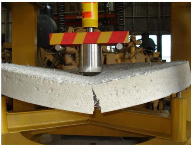
Fig. 5. Round panel being tested showing the flexural crack and the exposed synthetic fibers continuing to carry load.
