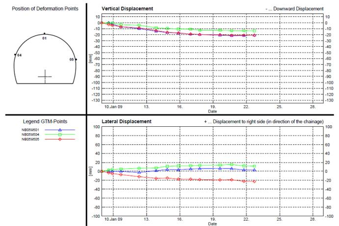
Fig. 12. Convergence measured during top heading excavation of the NB tunnel showing 15 to 20 mm of vertical and lateral displacement.
