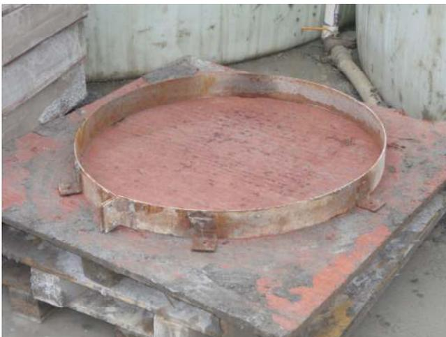
Fig. 10. Panel forms used at Devil's Slide for ASTM 1550 test.
