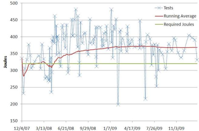
Fig. 11. Results of onsite ASTM 1550 testing at Devil's Slide Tunnel showing individual tests and the running total average.
