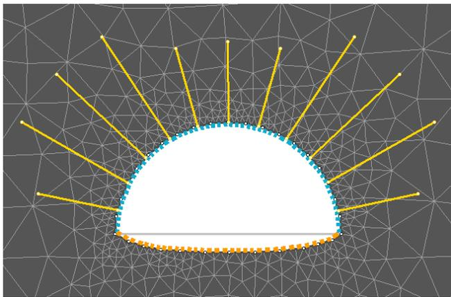
Fig. 13. Excavation and support after running through five stages of finite element model.
