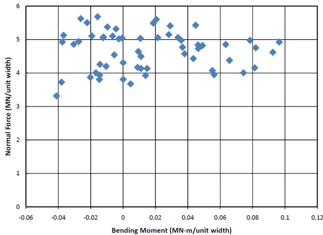
Fig. 16. M-N chart for the FRS top heading lining showing the axial and moment loading.
