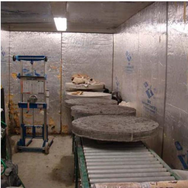
Fig. 9. Curing room with conveyor system for storage and handling of panels.
