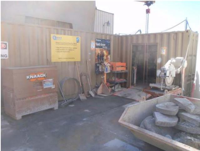
Fig. 8. Devil's Slide Tunnel Project onsite shotcrete and concrete testing facility.
