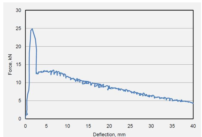
Fig. 7. Typical load vs. deflection curve for the synthetic fiber reinforced shotcrete at Devil's Slide.
