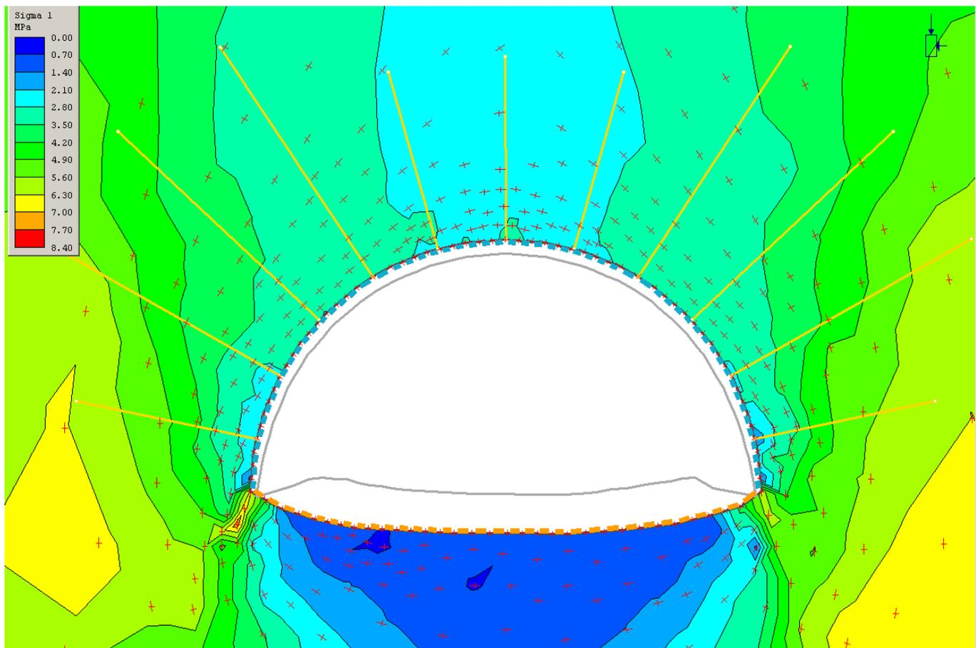
Fig. 15. Back analysis after Stage One showing  $\sigma_1$  contours, stress trajectories, and exaggerated FRS liner deformation.
