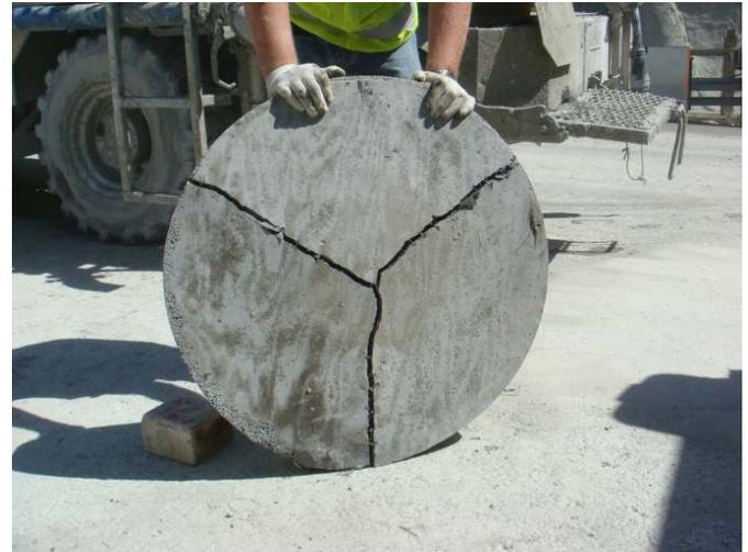
Fig. 3. Round Panel sample after testing.
