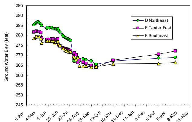
Figure 13: Ground water levels recorded by the piezometers on the East side of Taxiway F excavation.
