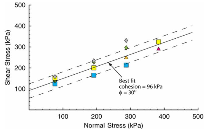
Figure 4: Summary of bedding plane shear strengths measured in direct shear tests on core samples. All samples tested exhibited a discrete open bedding plane
