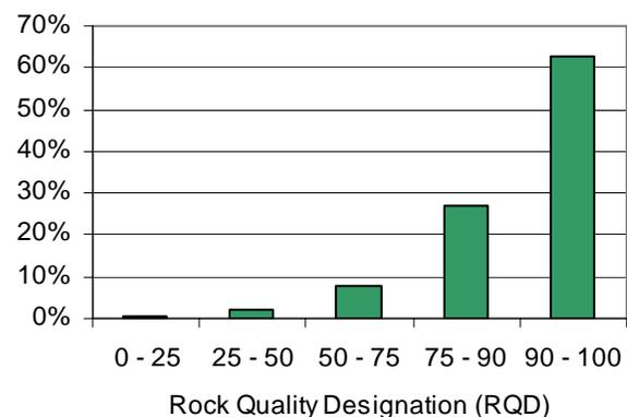
Figure 2: Rock Quality Designation (RQD) determined from various boreholes from the site investigations for the Dulles Airport rock excavations.
