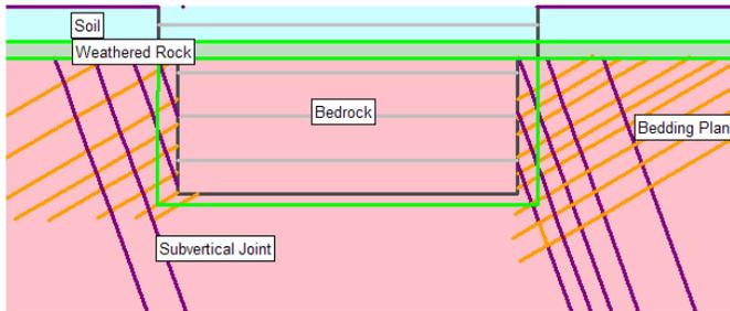
Figure 7: Phase2 model used to simulate the rock cut. The left side of the model is West and the right side
