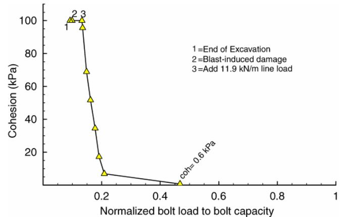
Figure 10: The reduction in cohesion along the bedding planes and the corresponding load increase in the anchor bolts from the numerical analyses.
