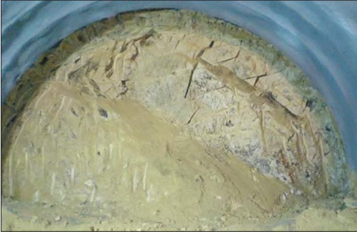
**Figure 8. Piedmont residual soil displaying blocky nature**
