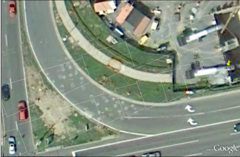
**Figure 2. View of International Drive ramp showing outline of tunnel sawteeth and location of CPT tests in the shallowest area over the tunnels**
