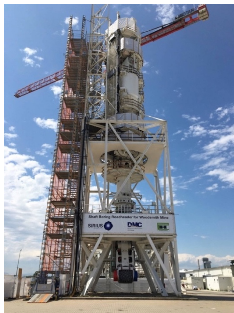
Figure 2. Herrenknecht shaft boring roadheader (Courtesy of DMC Mining Services).
