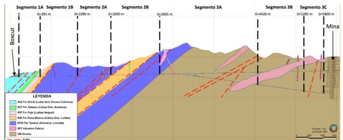
Figure 2. Geotechnical Segments along Tunnel Alignment.
