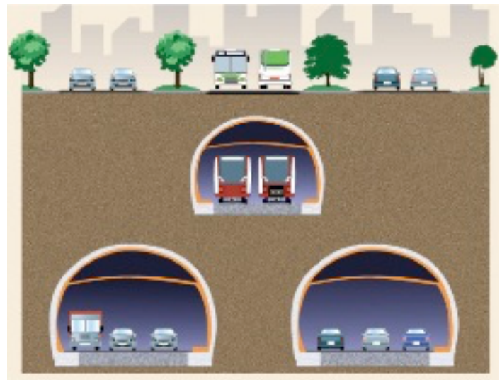
Figure 1. Schematic design of AVO II tunnels under Metro's Line 4 (Courtesy of Chilean Ministerio de Obras Publicas).
