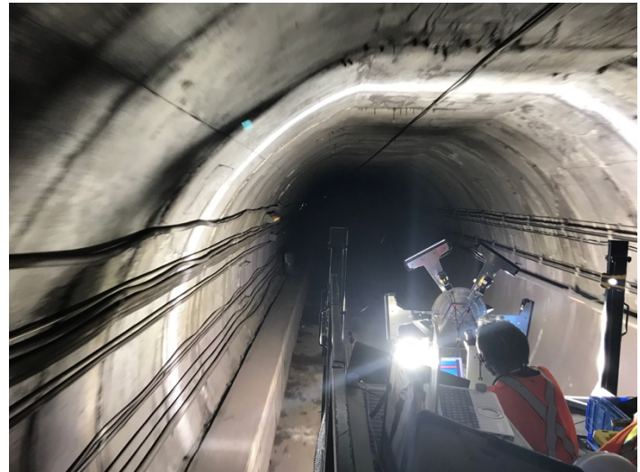
Figure 2. Tunnel photographic and thermographic scan performed from high rail vehicle.
