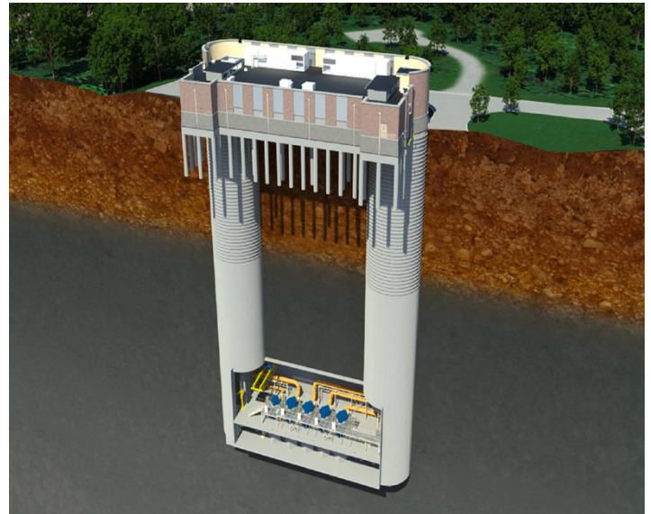
Figure 2. Pump Station Structure (Courtesy of MWH).
