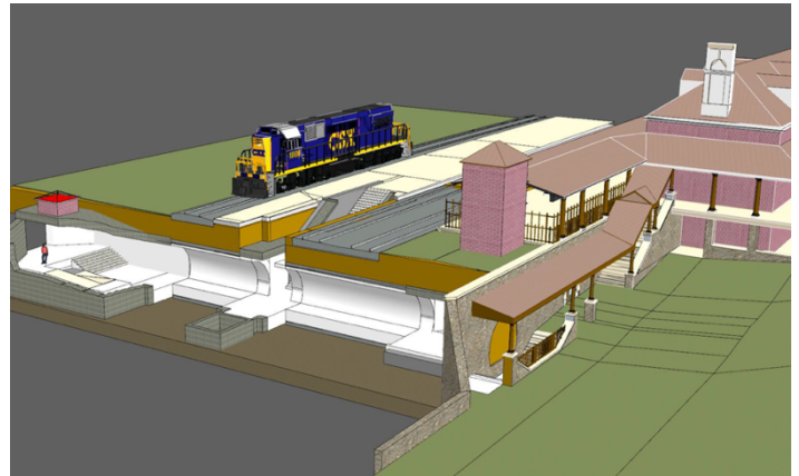
Figure 2. 3D rendering of Alexandria Station showing proposed pedestrian tunnel beneath the active rail lines.
