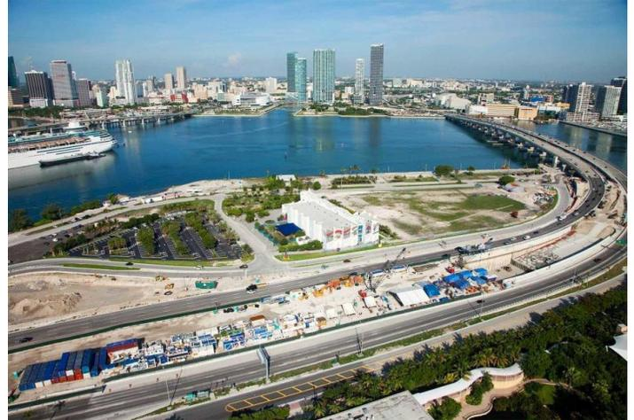
**Figure 1.** West Portal and Eastbound TBM launch location on Watson Island. (Courtesy of FDOT)
